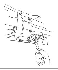
Thread supplied bolts 2x (9) into Front Drive Linkage. Repeat step for Rear Idler Linkage. Do not tighten.
