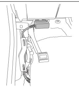
**OBD II install:** Use Supplied Posi-Lock™ connectors to attach the Plug and Play Module to the Harness. Attach matching colors on the harness to the wires on the module. Plug in module to OBD II port on the vehicle. Secure harness with supplied tie wraps. *Note: If the OBD II pass thru harness (76404-01A) was purchased see install sheet supplied in packaging. The pass through harness allows for an open port for other accessories. See below for a brief description.*
