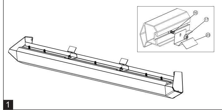
Using Flange Nuts (17), assemble Brackets 2x (25) & 1x (26) onto the rail (4), using the carriage bolts (16) left from previous step. Next, install Flange Bolt (14) and Flange Nut (17) onto bracket tab. Driver side shown. Dimensions shown are for reference.
