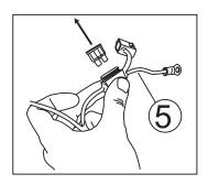
Attach wire harness to controller (make sure connector locking tabs fully engage). Mount controller with the two 11" tie wraps (20) to factory conduit, just forward of
