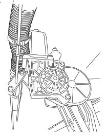
Torque bolts on mounting brackets to 16ft-lbs.
